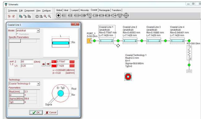
Fig. 4: Dialog box for setting and editing component parameters.
