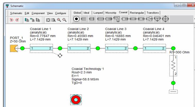
Figure 3: Chebyshev 4-section transformer's scheme with Coaxial palette shown.
