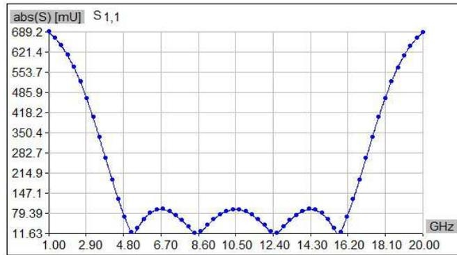
Fig. 5: Reflection coefficient (S11 parameter) magnitude.
