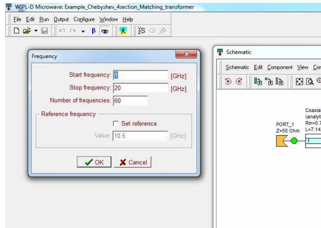
Fig. 2: Dialog box for defining a frequency range in a microwave circuit simulation project.
