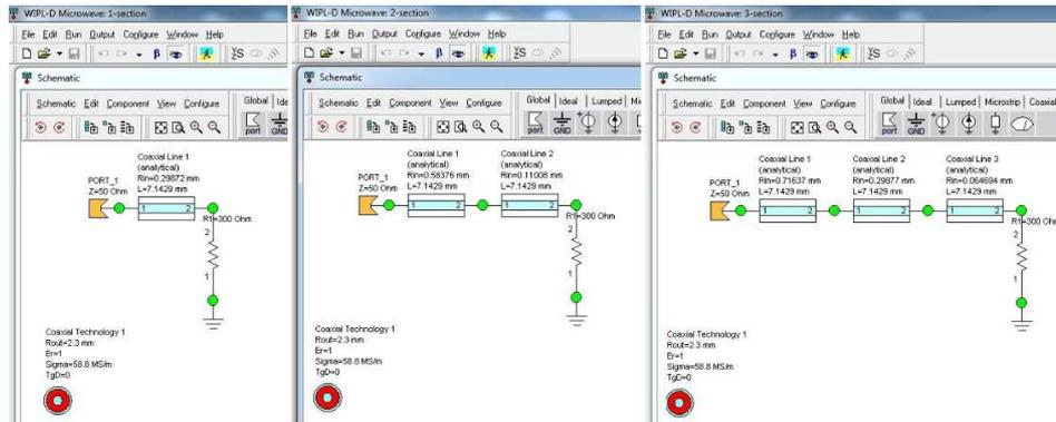
Fig. 7: Chebyshev 1-, 2-, 3-section transformer's schematic.
