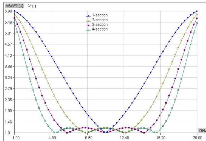
Fig. 9: VSWR comparison for Chebyshev 1-, 2-, 3- and 4-section transformer.
