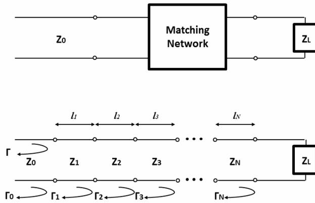
Fig. 1: Multisection matching network; general form with reflection coefficients.
